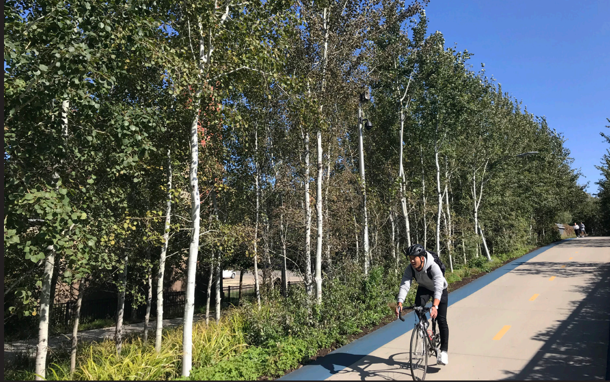
Material changes convey information: along the main circulation route of the 606 in Chicago, Illinois (MVVA), strips of blue rubber indicate jogging lanes while marks on the pavement indicate bike lanes. (Property of author)
